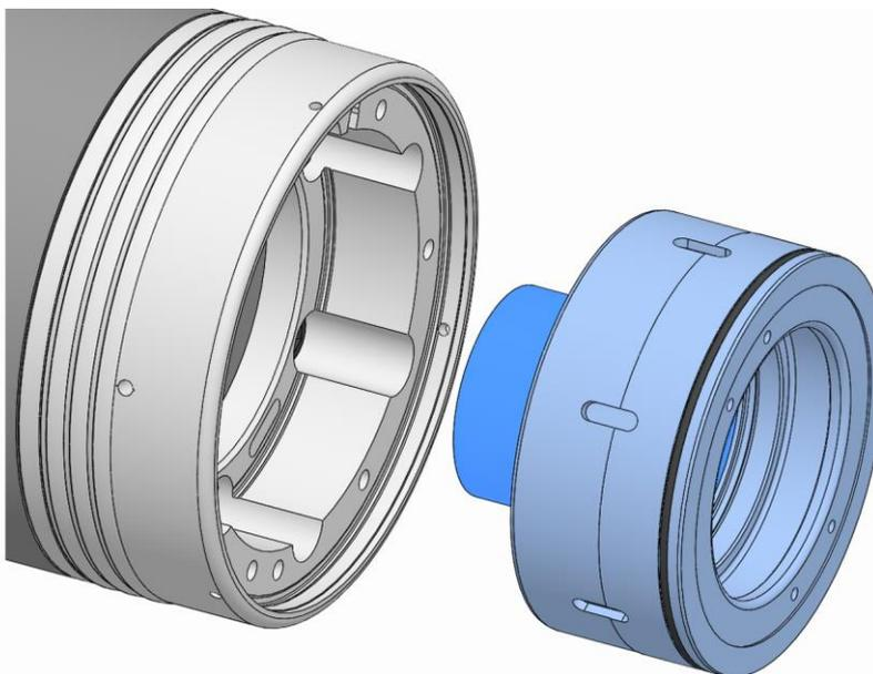
4. If necessary, screw the coupling and drawtube adapter firmly home on the machine drawtube.
