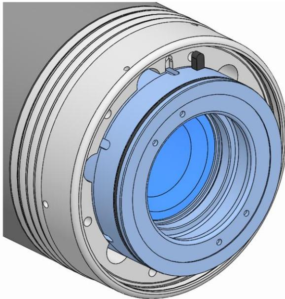
7. Install the coupling anti-twist device vertically in the base of the coupling groove, then press it into the groove in the spindle flange.
