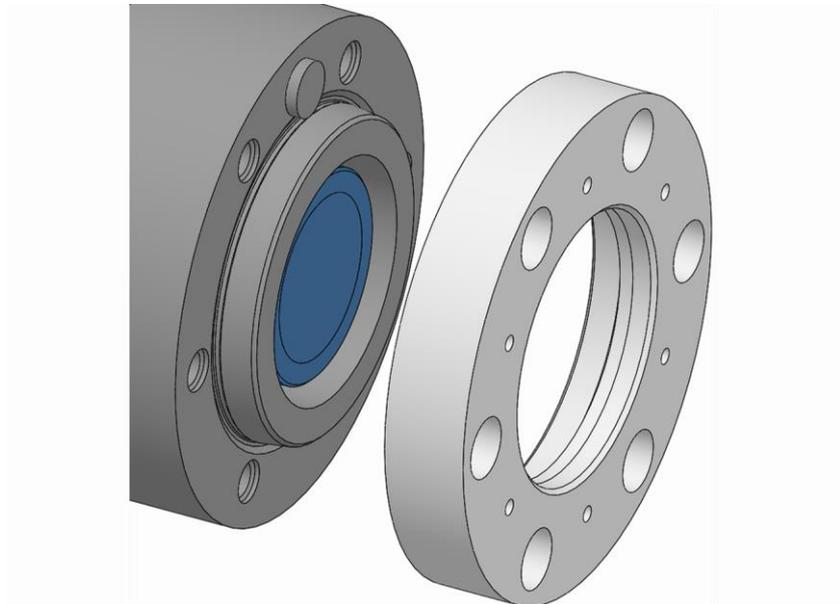
4. Take down the spindle flange from the machine spindle.
