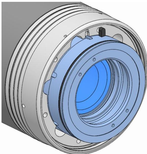
6. Remove the coupling anti-twist device from the coupling groove and the groove in the spindle flange.
