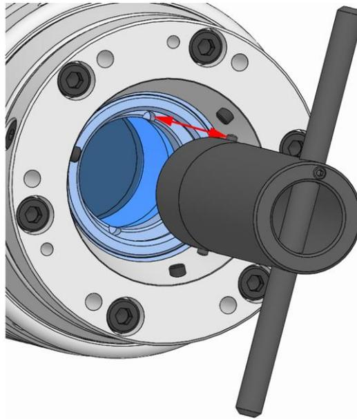
1. Insert the wrench for installing the reducing coupling in the product. For this, the pins of the installation wrench on the reducing coupling must be aligned with the grooves in the reducing coupling.
