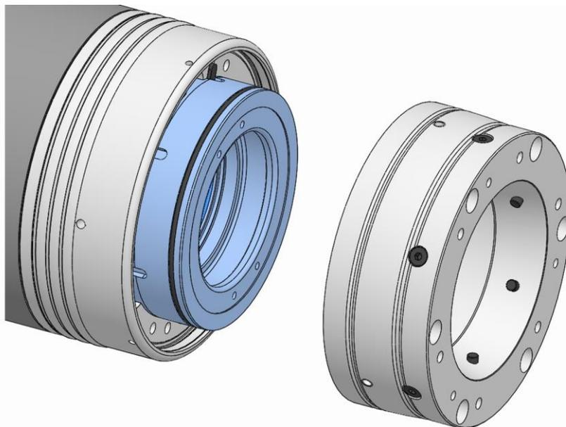
5. Take down the clamping element receiver from the spindle flange.
