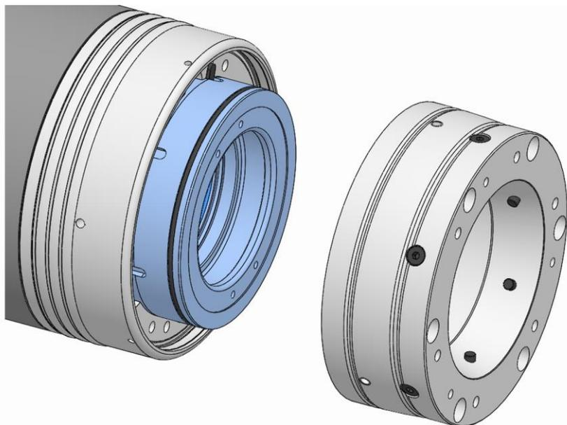
8. Fit the clamping element receiver on the spindle flange with the grooves in clamping element receiver and anti-twist device aligned with one another.
