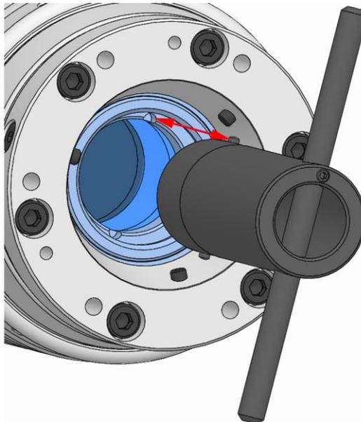
2. Remove the wrench for installing the reducing coupling.
