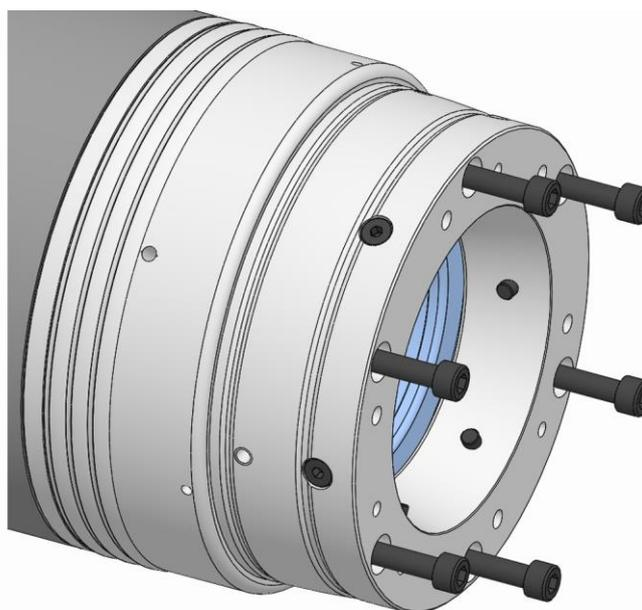
9. Screw in the clamping element receiver fixing screws and tighten them to the specified tightening torque [see »Screw tightening torques« chapter].
