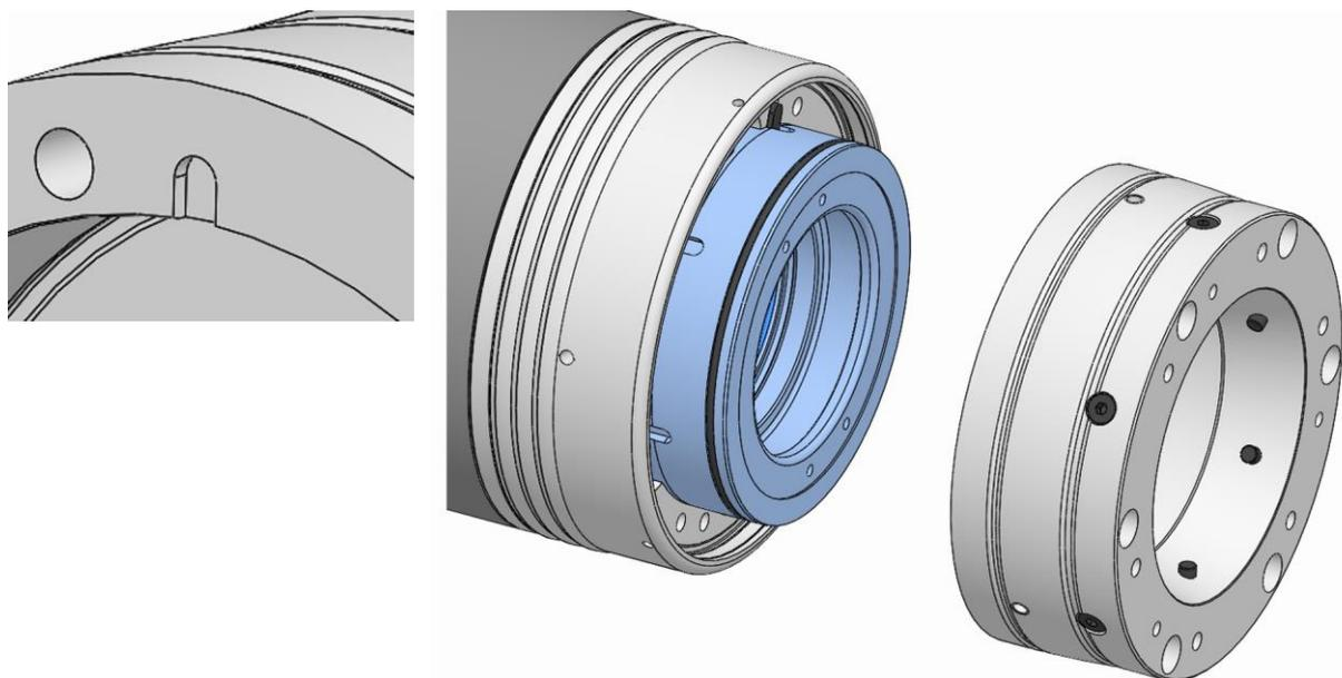
8. Fit the clamping element receiver on the spindle flange with the grooves in clamping element receiver and anti-twist device aligned with one another.
