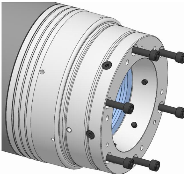
4. Unfasten and remove the fixing screws on the clamping element receiver.
