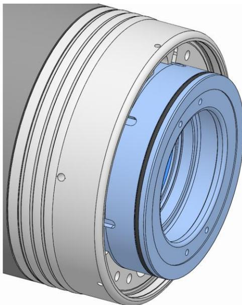
5. Rotate the coupling backwards until the next groove in the coupling and the groove in the spindle flange are aligned.
