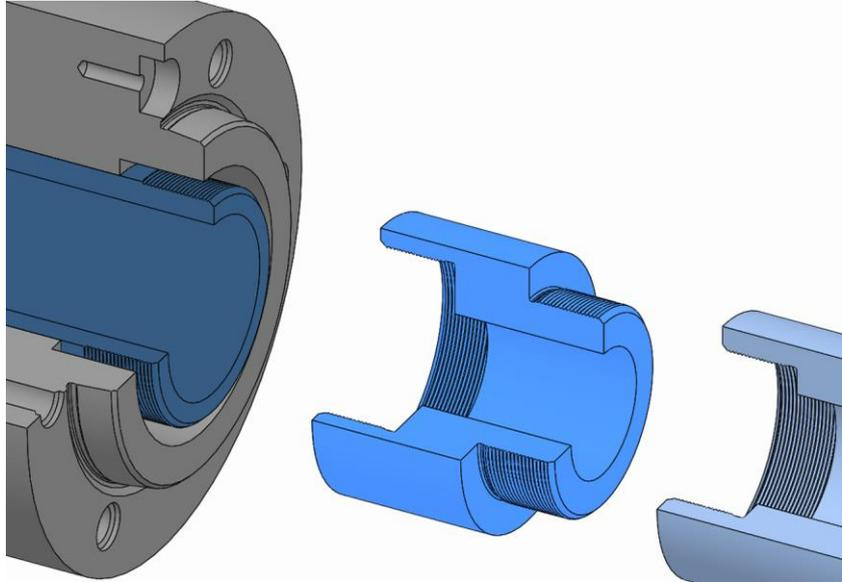
1. Screw the drawtube adapter into the coupling using its thread or screw it to the machine drawtube and tighten it down.
