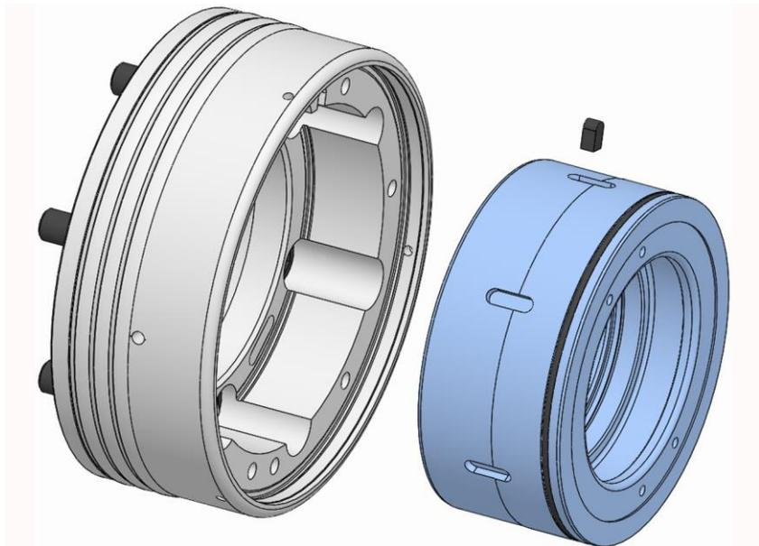
4. Remove the coupling and the anti-twist device from the spindle flange.
