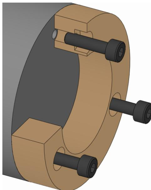
1. Unfasten and remove the fixing screws on the changing part.
