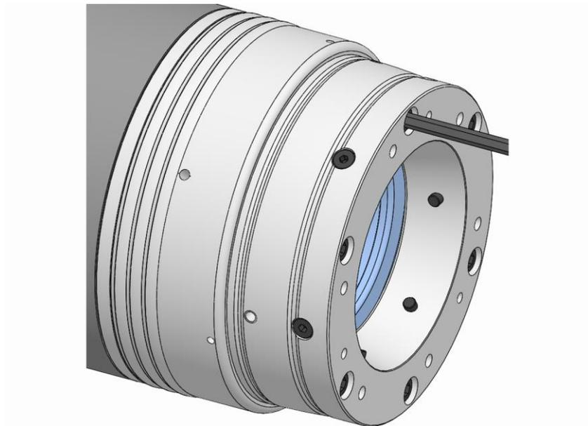
13. Tighten the clamping element receiver fixing screws to the specified tightening torque [see »Screw tightening torques« chapter].
