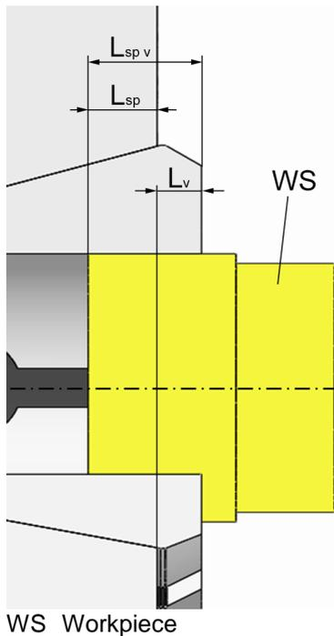
The clamping length is calculated as follows:
