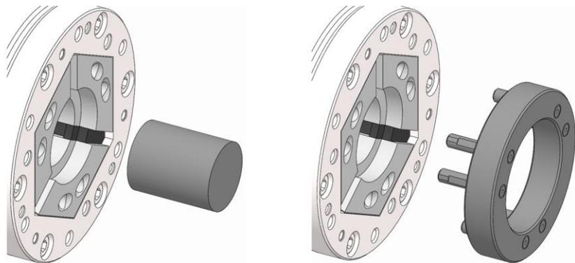
6. Remove the dressing pin from the clamping device. And/or remove the dressing ring from the HSW clamping head.
