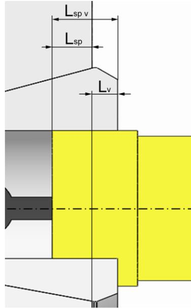
Without exception, never go below the total clamping length  $L_{sp\ v}$  of the workpiece, which measures at least 3 mm.
